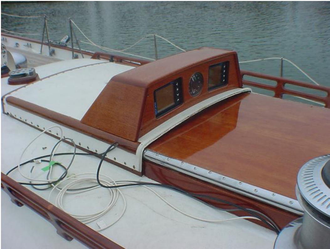
Ockam instruments are installed in an attractive teak box above the companionway hatch. The after portions of the grab rails include a second higher rail.
