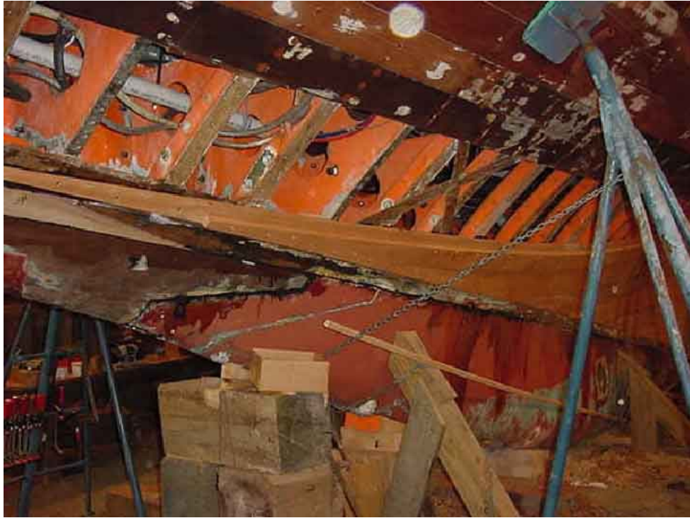
After replacement of the keel the new planks are installed. This view shows the bronze floors which connect the frames amidships, and the diagonal straps which reinforce the hull.
