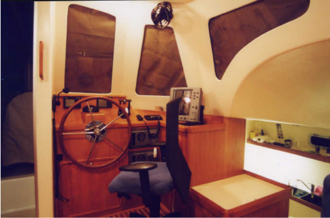
The inside helm. The dual steering systems are hydraulic and independent. The number of turns lock to lock is adjustable for each wheel, so it is easy to adjust helm pressure depending on sea state.
