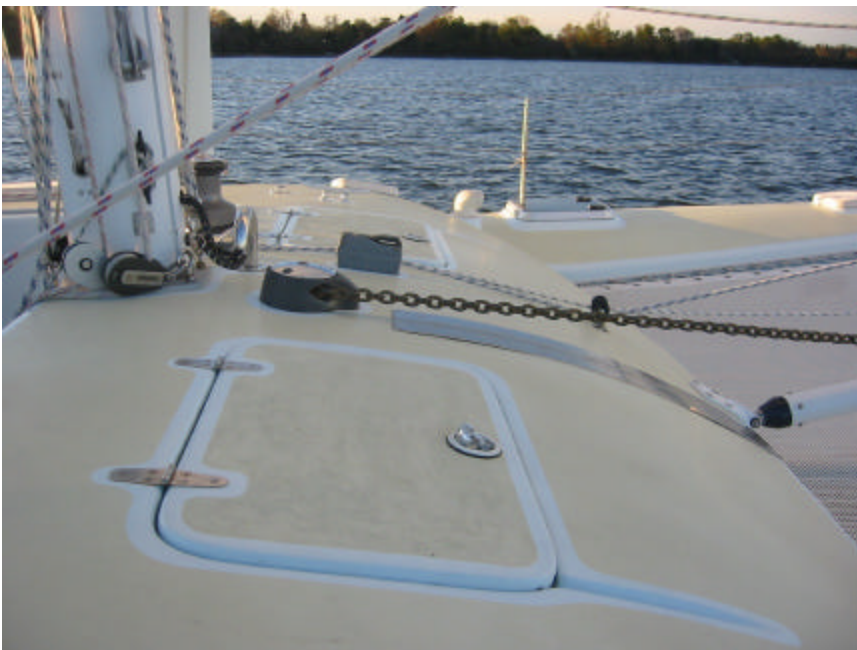
View across the foredeck shows the low-profile windlass and wing lockers.
