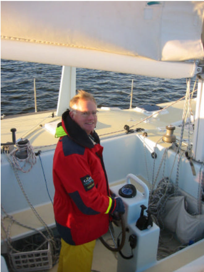
The outside helm includes dual-station engine controls and a VHF full-function remote microphone.
