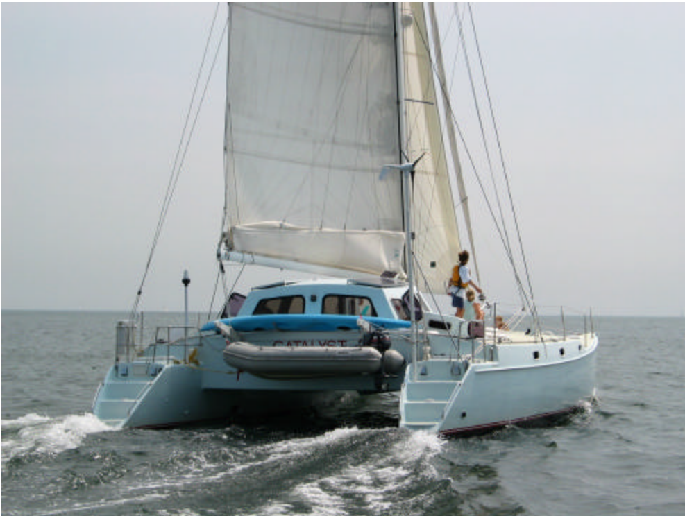
The dinghy (and here a kayak as well) store conveniently on davits between the hulls.
