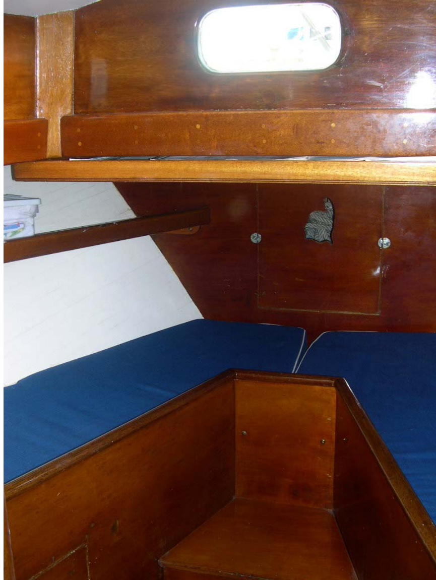
Forward "V" berth with drop-down chart tray under the forward deck. The anchor rode can be seen through the Indian-head cutout in the forepeak hatch. Storage lockers are located under the bunks.
