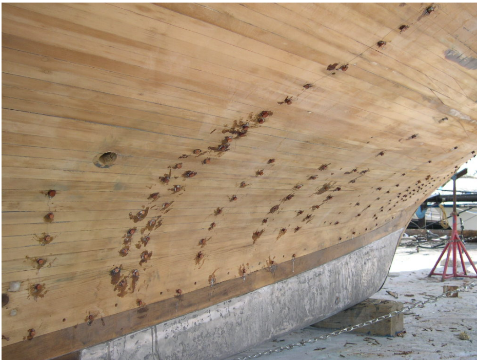
After 47 years the fiberglass below the waterline was removed, exposing the Alaskan cedar strip planking and lead ballast below the Greenheart keel. New stainless screws were installed and plugged as shown, and biaxial fiberglass was laminated with vinyl ester resin.
