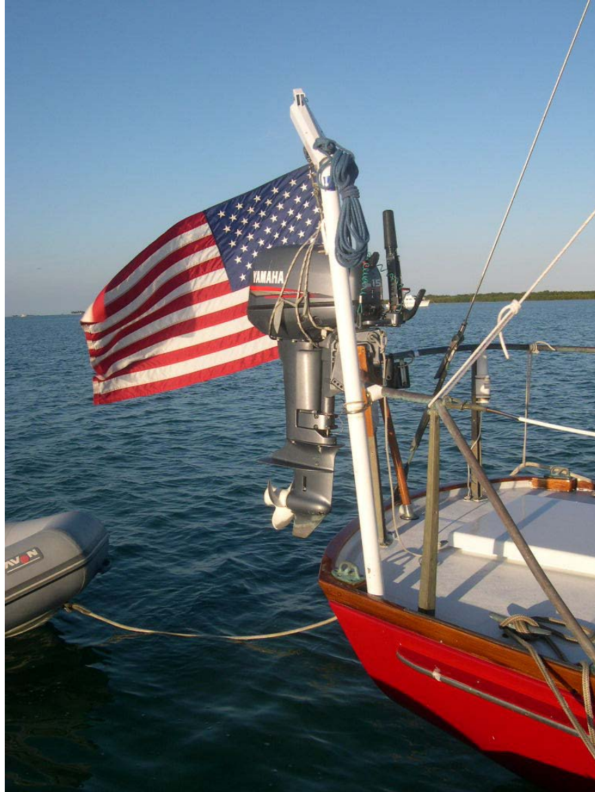
An outboard engine davit has made it much easier to lift the 15 HP engine to the carrying bracket on the aft pulpit rail. The davit can be removed and stowed when not cruising.
