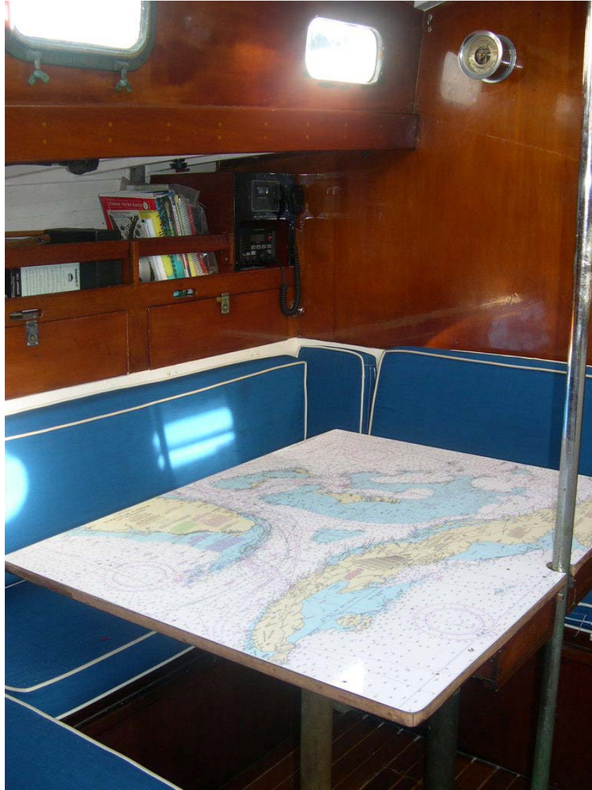
The salon table drops down to serve as a wide double sleeping berth when needed
