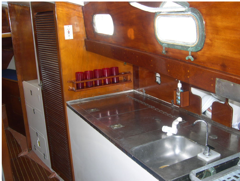
Galley area showing the ice box below the stainless counter top and the forward end of the gimbaled two-burner stove top.
