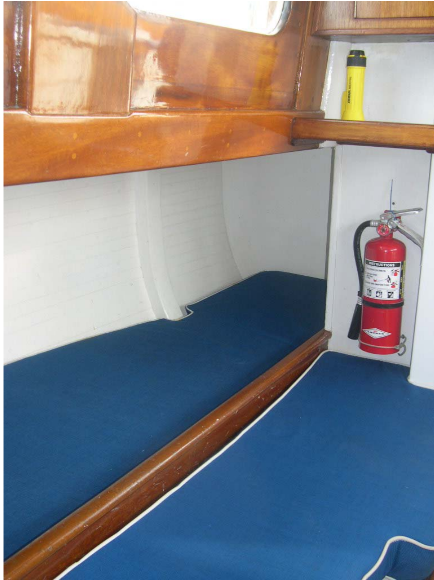
Comanche's starboard quarter-berth. An identical berth is on the port side. Inboard seat cushions on each side of the companionway step offer a place to sit out of the weather.
