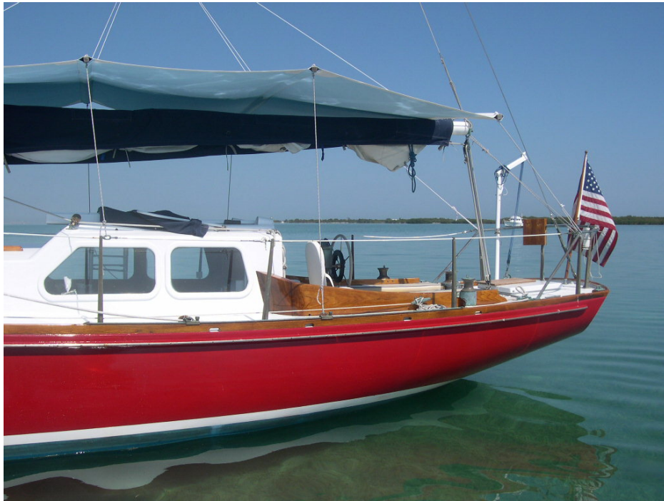
The large awning protects against sun and rain. The dodger is shown folded forward.
