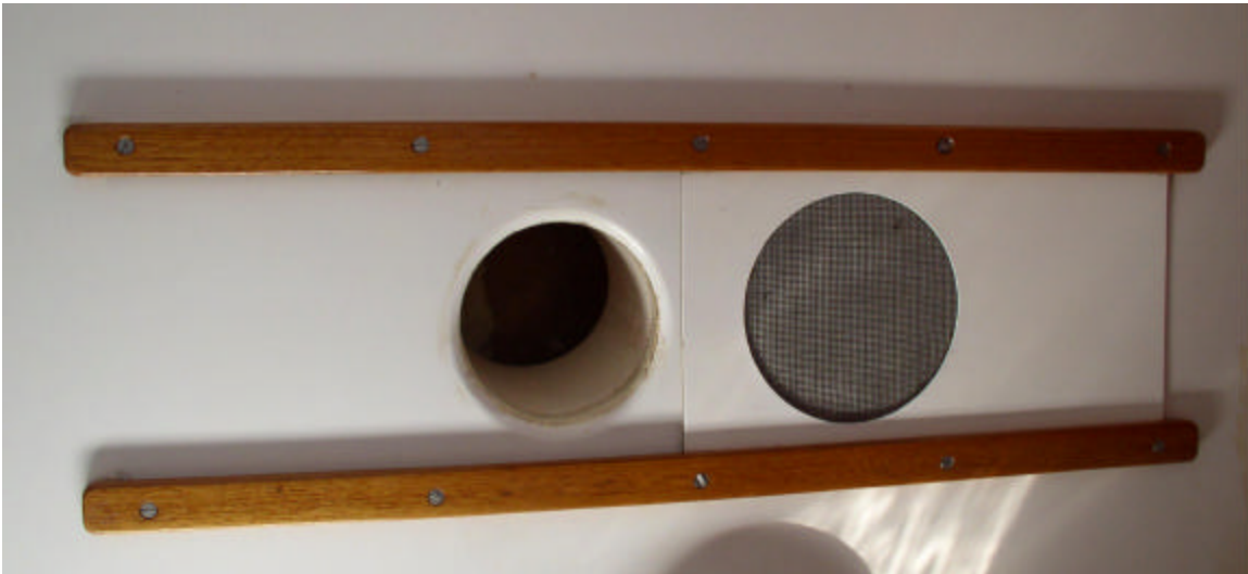
Sliding fiberglass panels are fastened to the overhead under the Dorade vents with three positions: open, screened, and closed.
