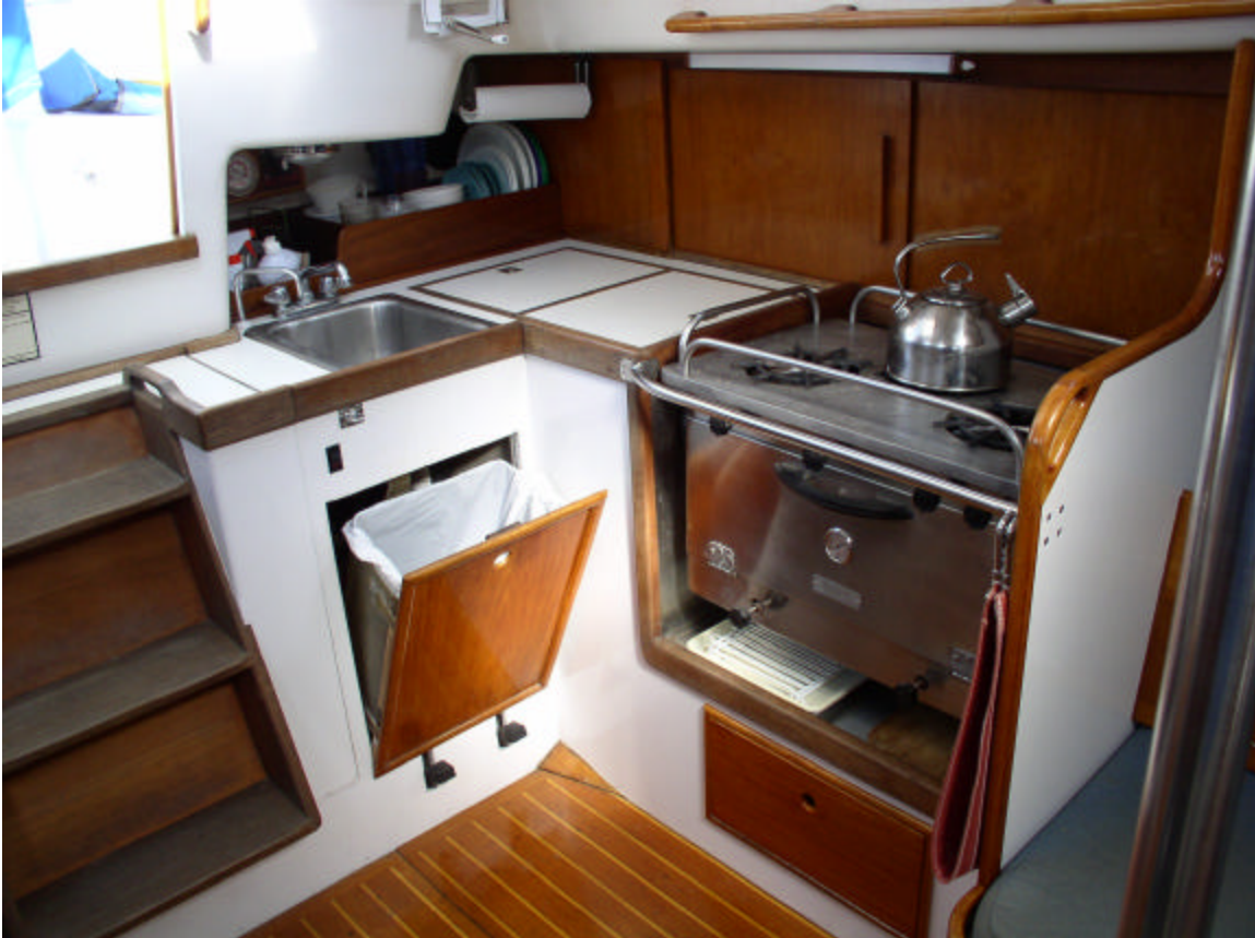
The Luke galley stove is gimbaled with a protective rail and strap for the cook. Dual footpumps under the trash locker are used for fresh and salt water, in addition to the pressure fresh-water system.
