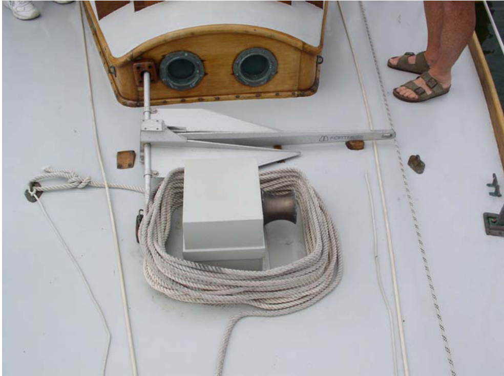
An electric windlass is housed in a special box on the foredeck. Ground tackle includes a CQR, the Fortress shown here, and two more anchors.
