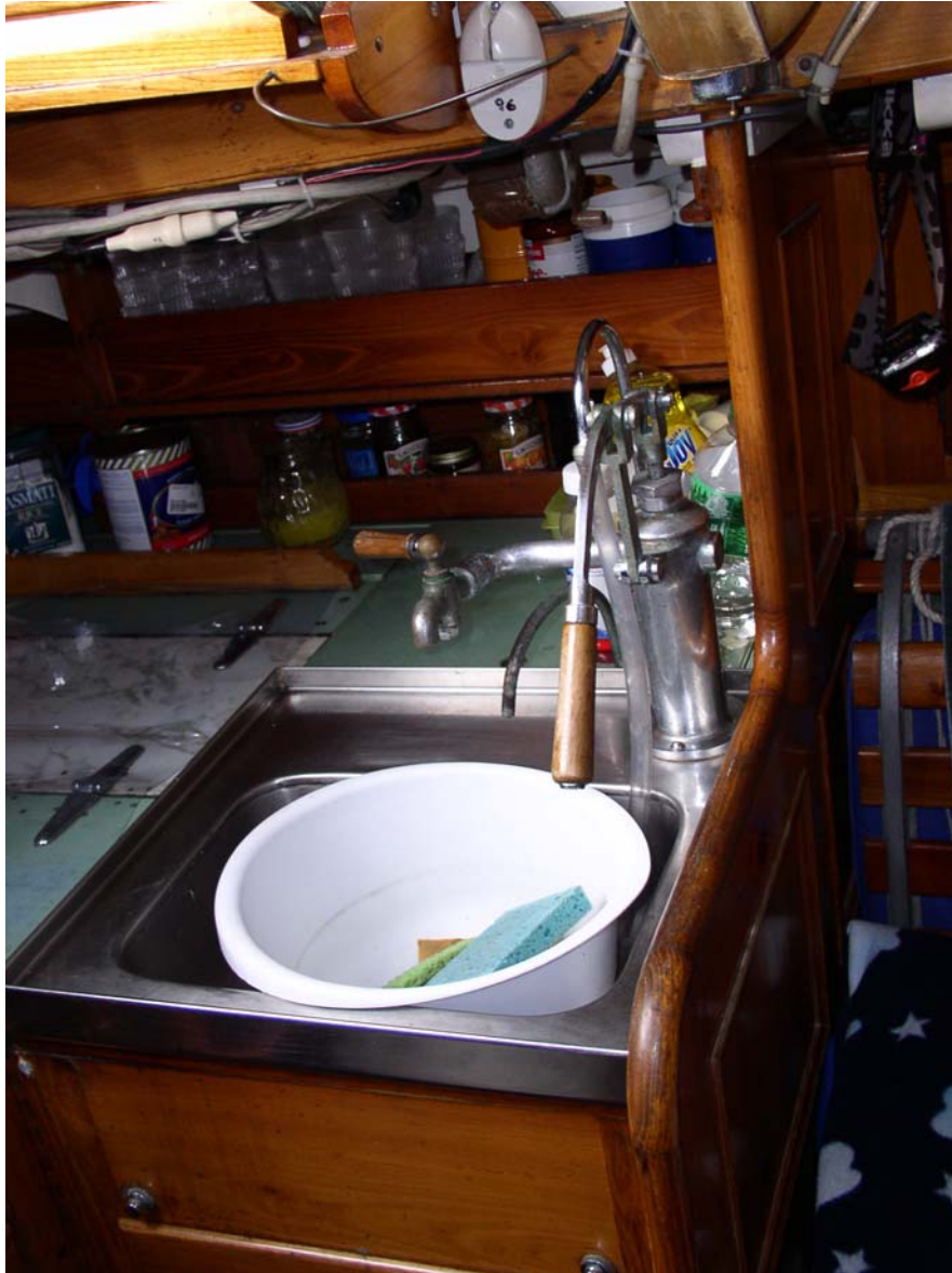
The port side of the galley includes a fitted stainless sink with a large manual pump. The faucet provides positive shut-off to conserve water. The ice box is refrigerated by a Sea Frost engine-drive compressor.
