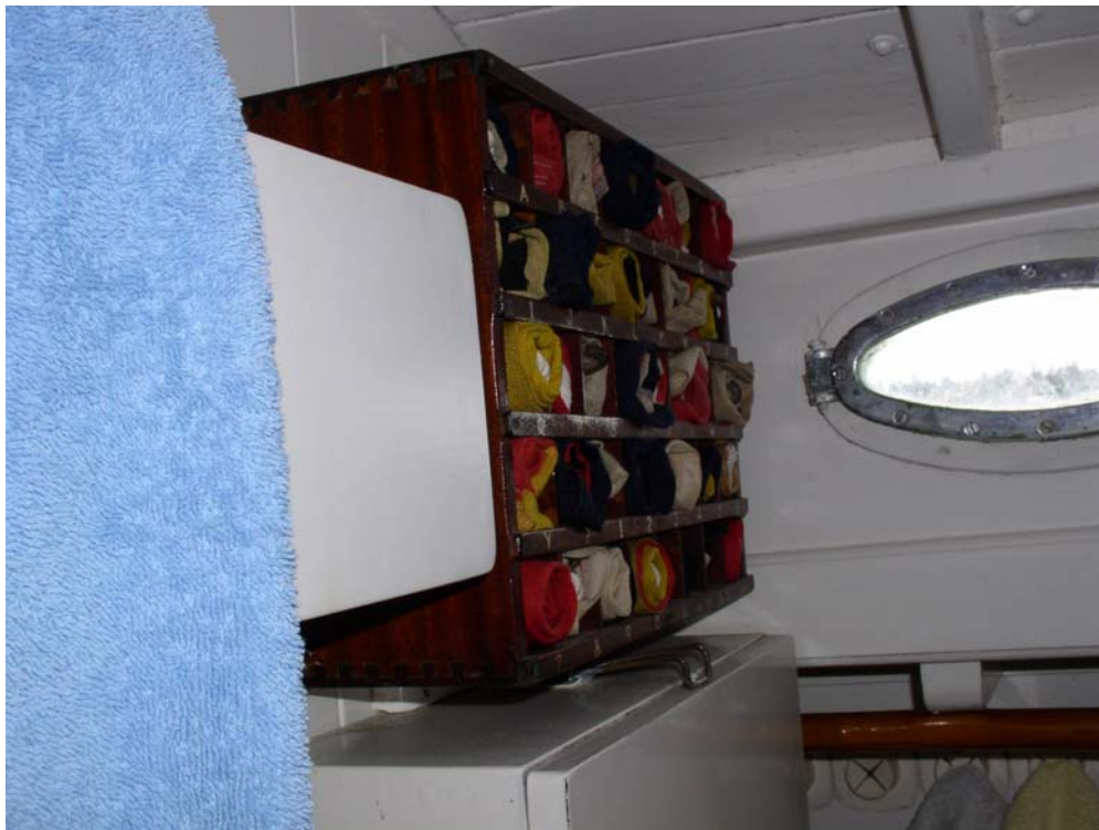
A proper locker for signal flags is mounted on the main bulkhead in the head.
