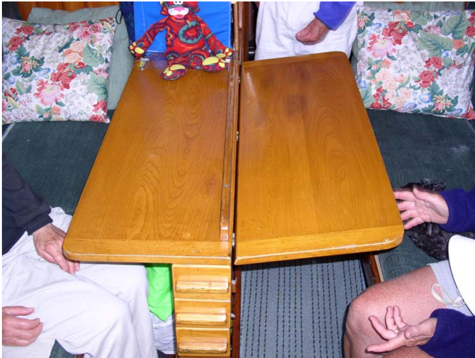
The leaves of the cabin table can be set at an angle to facilitate use offshore.
