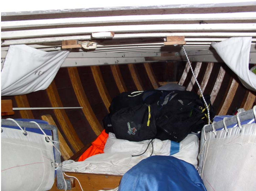
View of the forepeak and folding pipe berths in the forward cabin. The hull is planked with mahogany over laminated oak frames.
