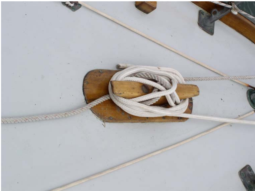
The Concordia cleats are made of locust. The decks are covered with canvas.
