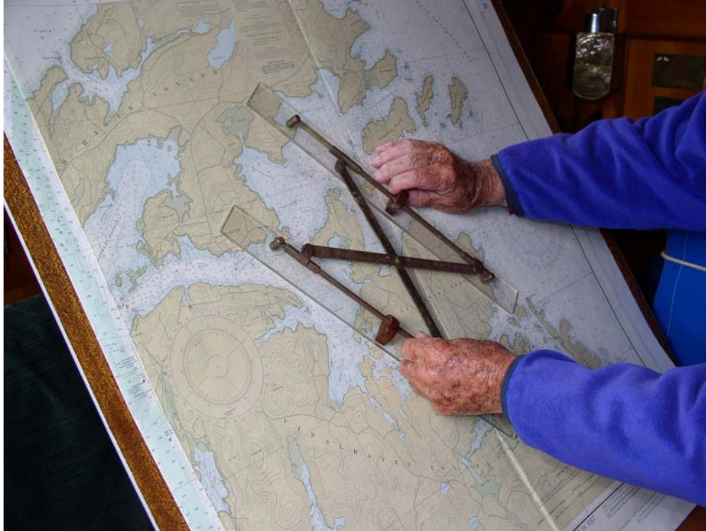
The owner has designed and built numerous fittings and equipment. This parallel rule has an extended width which minimizes the number of separate steps required to use it.
