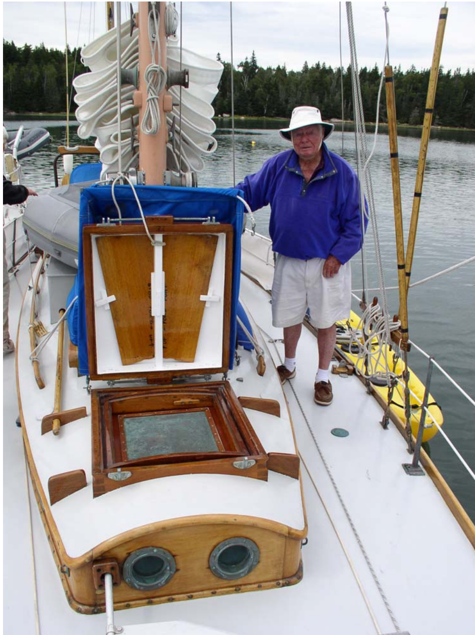
The forward hatch is one of the owner's many special creations. Hinged either fore or aft, it is supported on the sides by the quadrilateral panels to provide a strong sprayproof arrangement when open.
