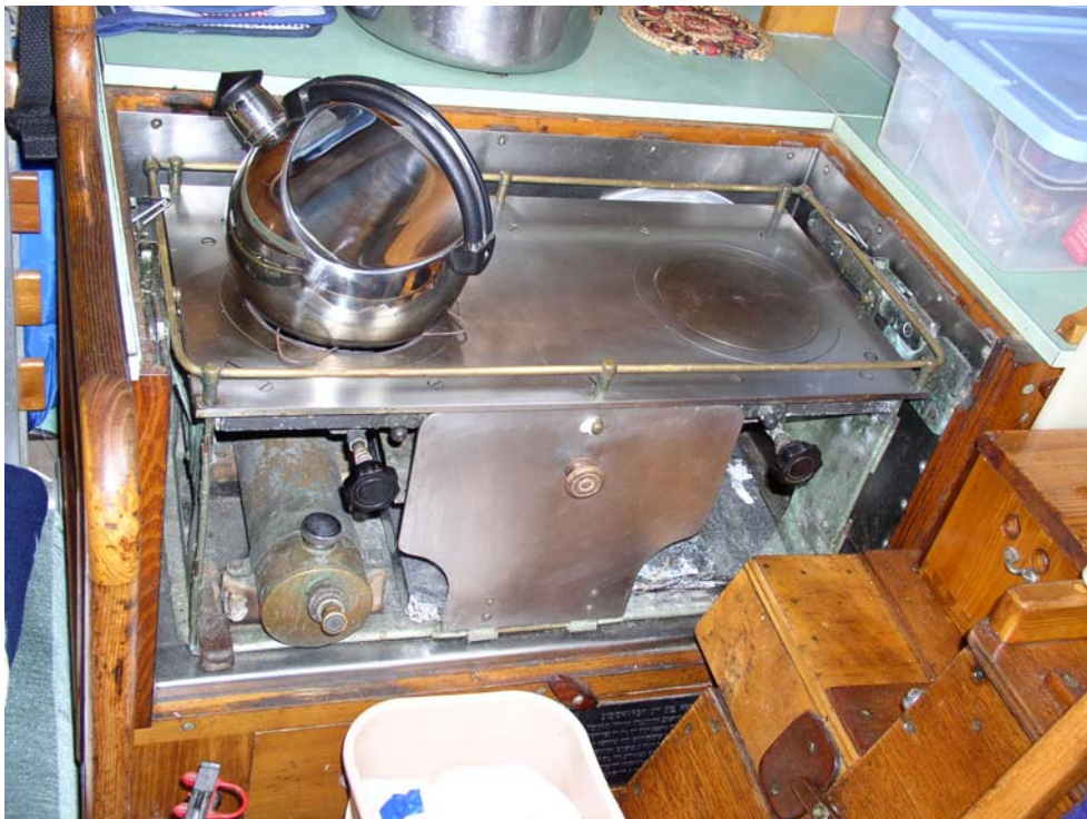
The gimballed alcohol stove is mounted on the starboard side of the companionway. The integral tank is filled by a special hose with gravity feed from a larger tank aft.
