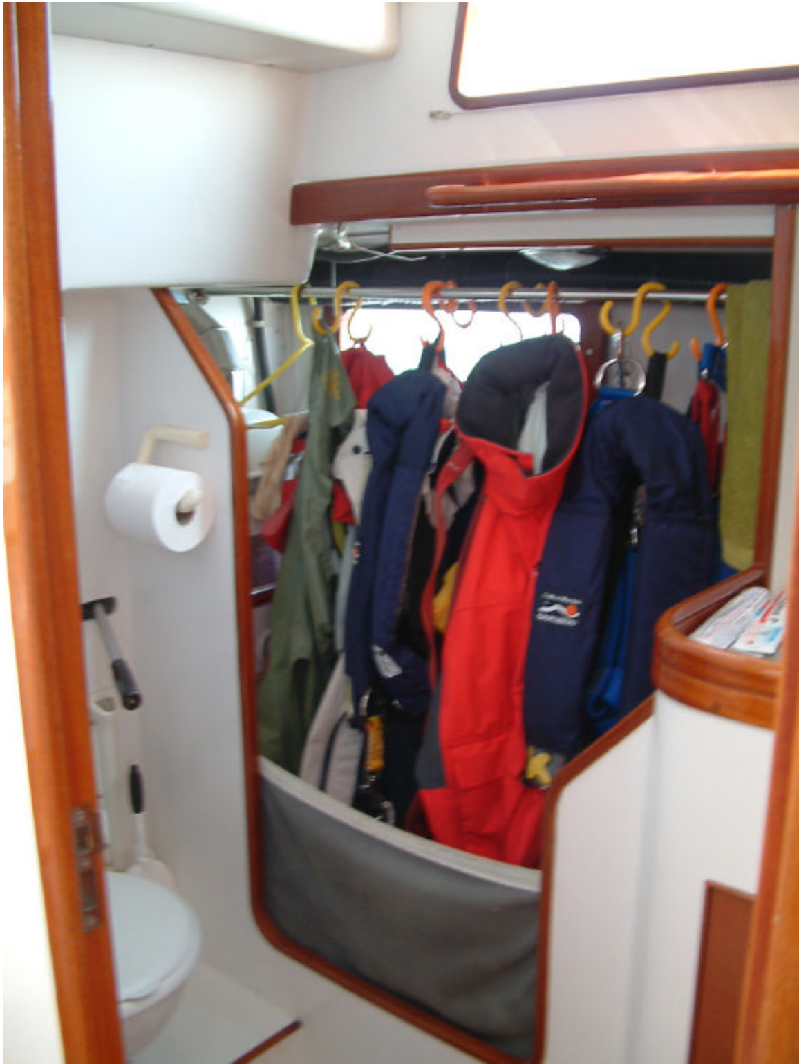
A substantial wet locker is outboard in the head, located immediately to port at the base of the companionway. Both the head and the landing below the companionway have draining teak grates on the sole; water from soggy crew members stays in this area and out of the pilothouse.
