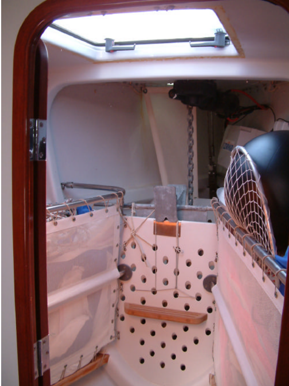
The forepeak is forward of a 3-latch watertight door. Two pipe and fabric bins hold spinnakers and other gear, while two anchor rode lockers are forward. Chain bin is deep vertically, to allow jam proof stacking under windlass. Spare Danforth anchor hangs behind chain pile. Fabric divider keeps rope rode all the way forward.
