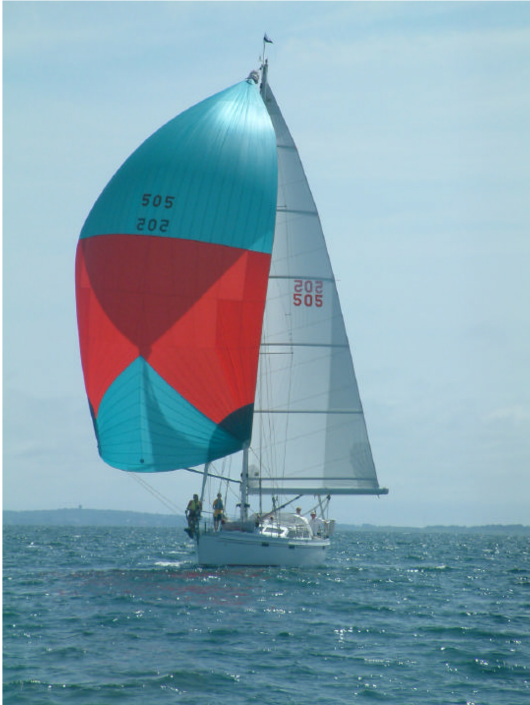
The large chute pictured is used downwind. An asymmetric also can be flown off bowsprit pole for reaching.
