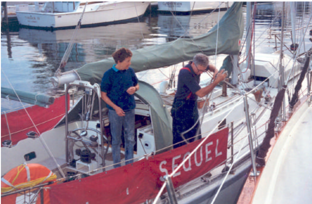
This photo shows Sequel departing for her circumnavigation. The dinghy stows in two halves on the foredeck. Both the staysail and yankee are set on Pro-Furl furlers. Twin headsails are used downwind, with a second yankee set from a wire-luff furler just aft of the forestay.
