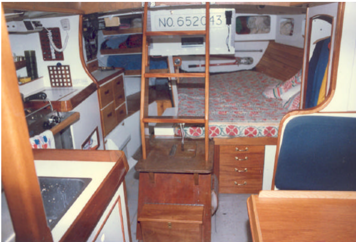
View looking aft shows the galley to starboard. To port is a double berth, with drawers for tools underneath. The engine is under the companion ladder.
