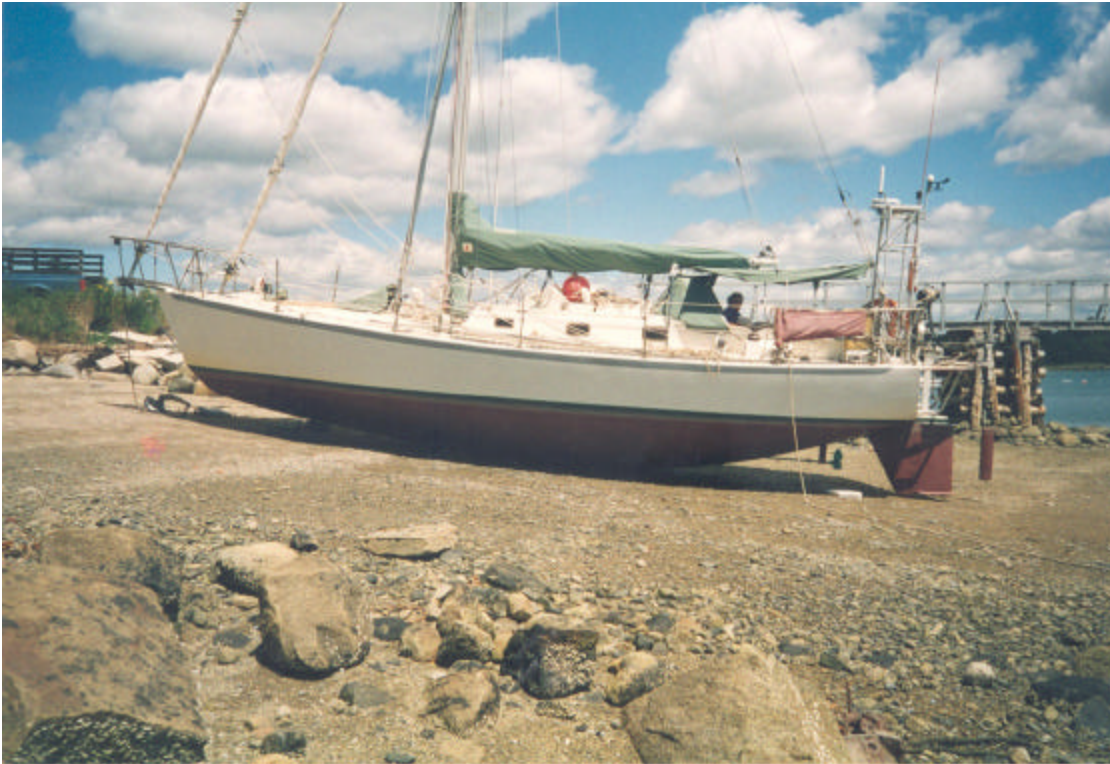
On the beach in Benjamin River, Maine, showing the original underbody/skeg-rudder configuration
