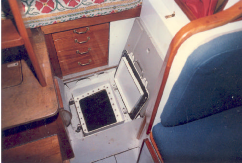
Alongside the companionway is a Lexan viewing port, protected by a gasketed hatch.
