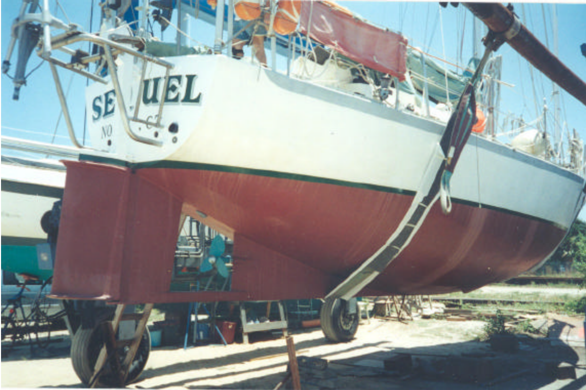
In slings after the underwater modifications were completed in 1997. The entire "keelet" and fixed skeg serve as a fuel tank, interconnected by the lower box girder. The 18" Max-Prop is well protected.
