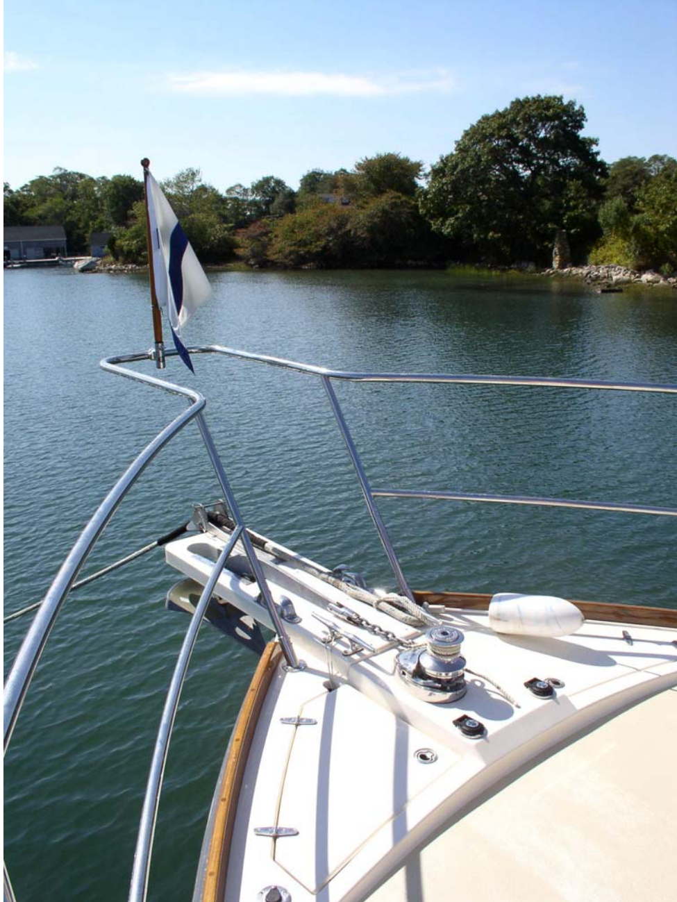
Ground tackle includes a Spade anchor and Lewmar windlass with up/down foot controls. Deep lockers are on both sides of the windlass. Fresh and salt water washdown receptacles are set flush in the deck outboard.
