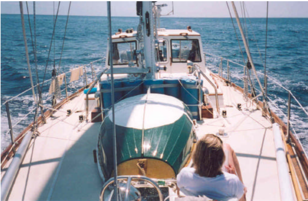
The dinghy is carried on the foredeck. It is inverted for offshore passages, as shown here in mid-Atlantic. The blue cannisters were used to carry extra fuel for the crossing. Note the husky guards over the Dorade ventilators, and the stainless hinged platform on the starboard guard which is used to reach the mainsail and halyards on the mast.
