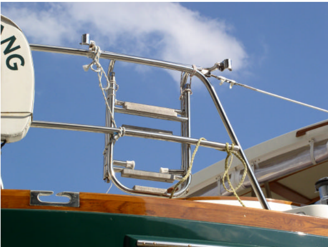
The boarding/swimming ladder is hinged in three sections. In use it is suspended from the stanchions by the upper clips. (See the next photo.)
