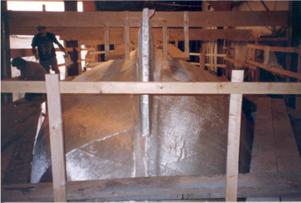
The hull was built inverted using four layers of 24-ounce biaxial E-glass on both sides of \frac{3}{4} inch Core-Cell foam.
