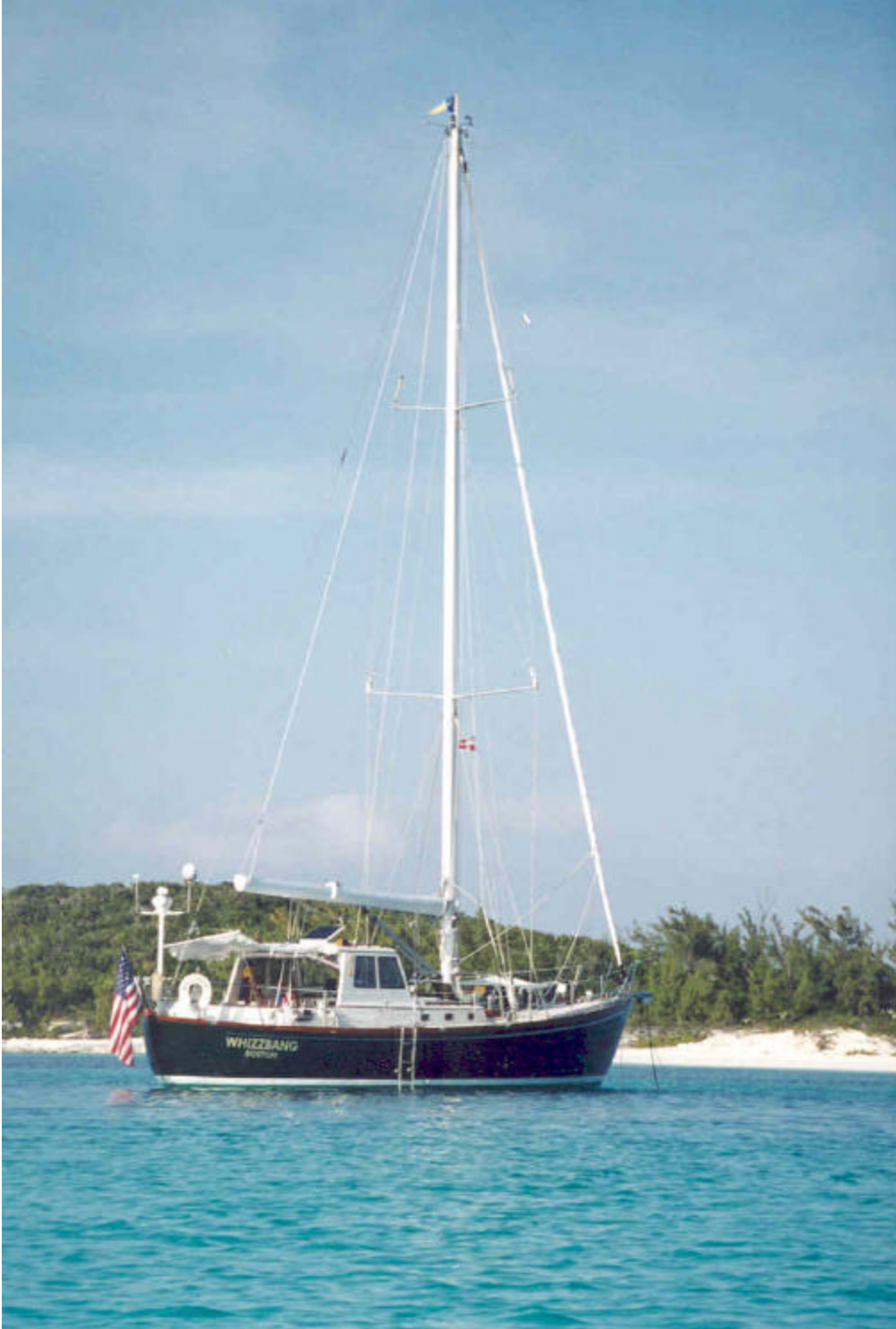
Whizzbang at anchor in the Bahamas. The canvas cockpit canopy is supported by the deckhouse roof and backstay, and it can be easily rolled and unrolled without detachment at the forward end.
