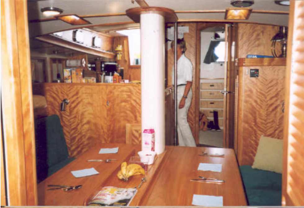
View looking aft shows the owner's cabin to port. The birch veneer is all from one tree. The stainless stanchion to the right of the mast houses the centerboard pennant, and serves as a convenient handhold.
