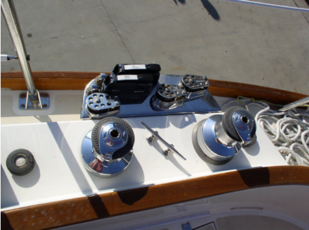
Lewmar #54 electric winches on the coamings are used with rope clutches and turning blocks for the headsail sheets and furling line.
