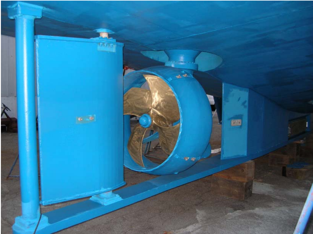
Aft compression post, hydraulic rudder, Z-Drive, and keel cooler. The Z-Drive can be rotated 360 degrees without unwinding, allowing for full power in reverse when rotated 180 degrees.
